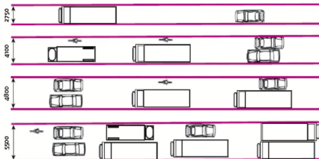
Figure 7.1 Illustrates what various carriageway widths can accommodate. They are not necessarily recommendations.
